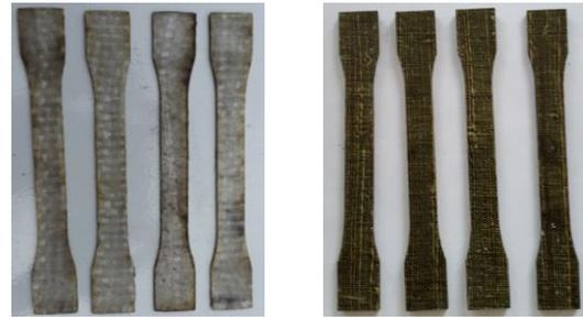
GAMBAR 4. Contoh spesimen uji tarik FG-FG-FG dan S-FG-S
