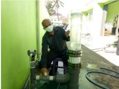
Gambar 5. Pengujian permeabilitas beton porous.
