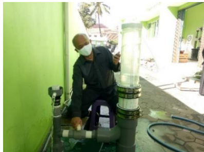
Gambar 5. Pengujian permeabilitas beton porous.
