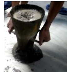
Gambar 5 Proses uji slump
