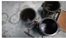
(c) silinder beton
