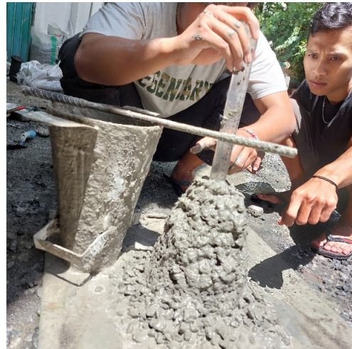
Gambar 5. Uji slump beton
