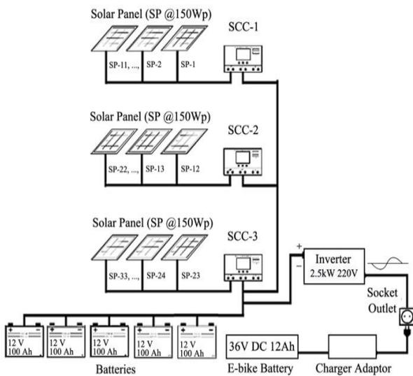
Fig. 3. Electrical design of a solar-powered e-bike charging station
