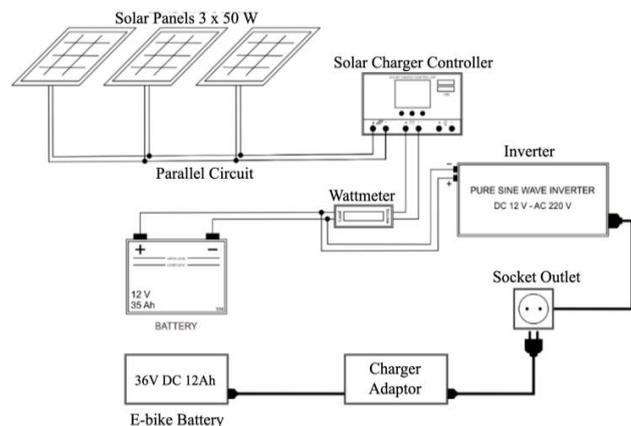
Fig. 2. Preliminary design of a solar power plant using 150 Wp solar panels with a capacity of 142 Wh
