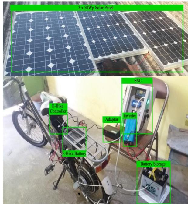
Fig. 4. Test setup of the proposed solar-powered e-bike charging station
