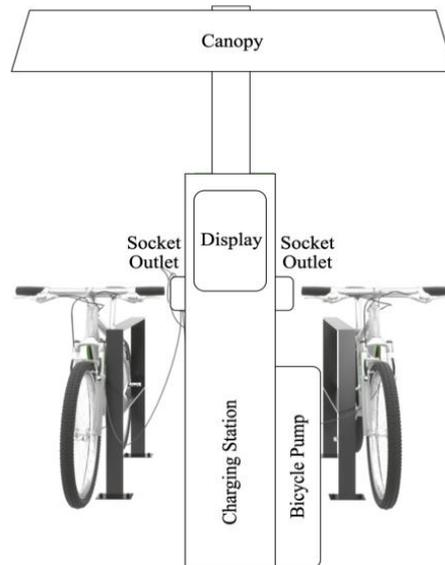
Fig. 1. Desain of charging station which is integrated with a bike parking lot
