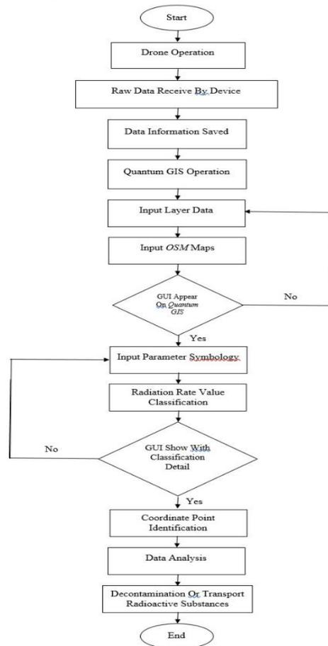
Fig 4. Drone Detection System Mapping Flowchart Using Quantum GIS
