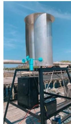
Fig 9. Savonius type wind turbine
