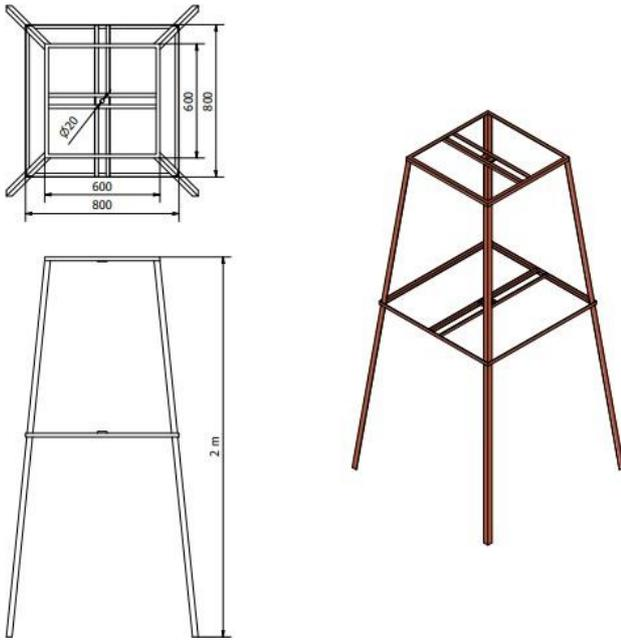
Fig 3. Wind turbine support frame design
