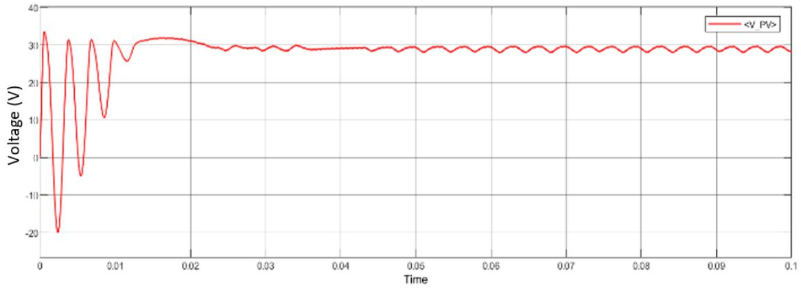
Fig. 4. Voltage of solar photovoltaic at 25 °C
