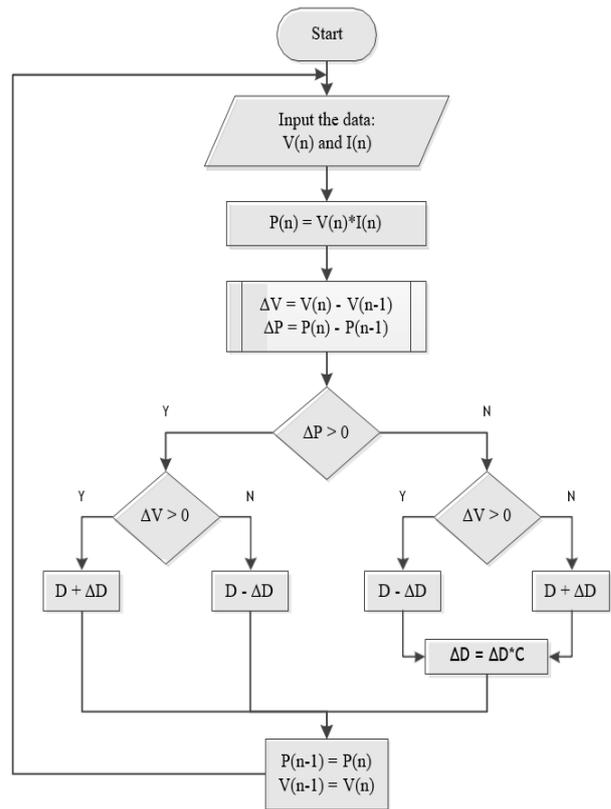
Fig. 3. Flowchart of the modified Perturb and Observe (PO) algorithm [6]
