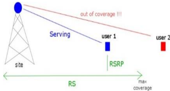
Fig. 2 Reference Signal Received Power (RSRP)
