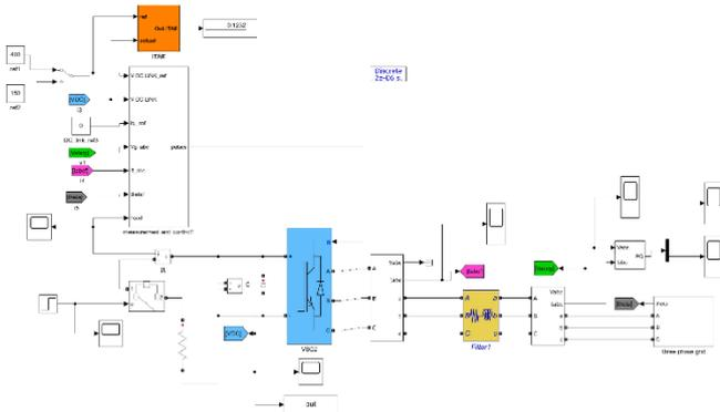
Fig. IV. Simulation of Active Rectifier System with PI-PSO Controller
