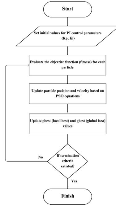
Fig. III. Flowchart of PI Controller Design with PSO Optimization Method
