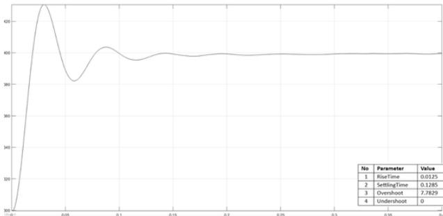
Fig. V. Actual Voltage with 100-ohm Resistive Load at Time 0 Seconds
