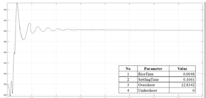
Fig. VIII. Voltage on a 100 Watt Constant Power Load at Time 0.25 Seconds
