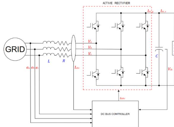
Fig. I. Block Diagram of Active Rectifier System
