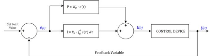
Fig. II. Block Diagram of Control System with PI Controller
