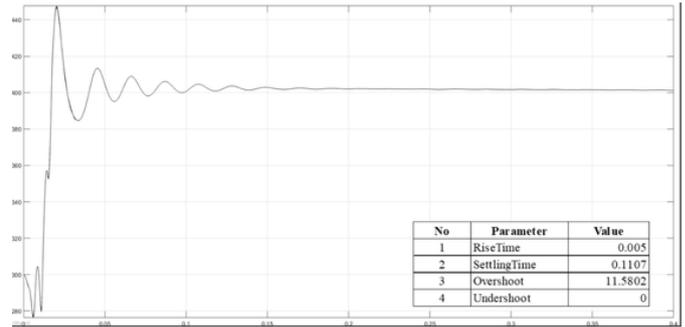
Fig. VII. Actual Voltage on a 100 Watt Constant Power Load at Time 0 Seconds
