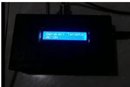
Fig 11. LED display when movement is detected by the radar sensor, prompting the air conditioning unit to turn on immediately
