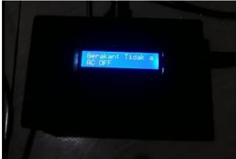
Fig 9. LCD display no movement AC becomes off
