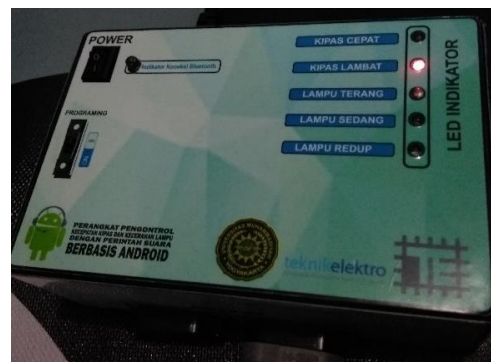
Fig. 10. LED indicator when the fan is slow
