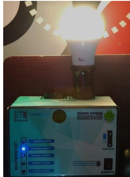
Fig. 16. LED indicator when the light is medium
