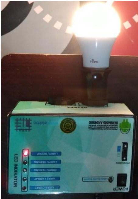
Fig. 18. LED indicator when the light is dim
