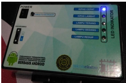
Fig. 7. LED indicator when the fan is fast
