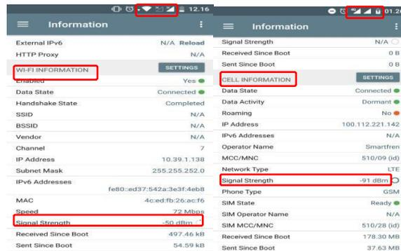
Fig. 7. RSSI LTE network and WiFi measurement results
