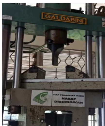
Figure 2. Universal testing machine Autograph Machine COM-TEN 95T Series 5K to bending testing
