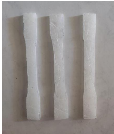
Figure 3 Specimens for Tensile Tests
