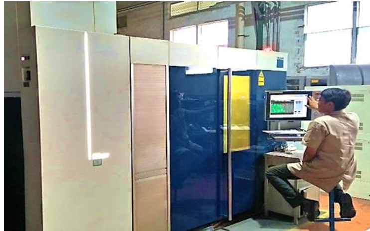
Gambar 1. Mesin Laser Cutting TruLaser 3030 Fiber (L49)
