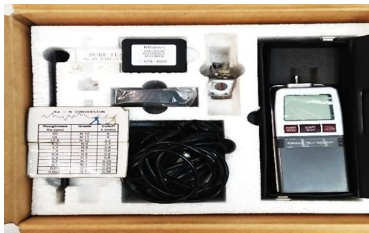
Gambar 2. Surface roughness tester merek Mitutoyo Type SJ-201P
