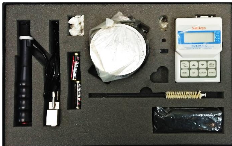
Gambar 3. Hardness tester merek Mitutoyo Hardmatic Type 810-299 HH-299
