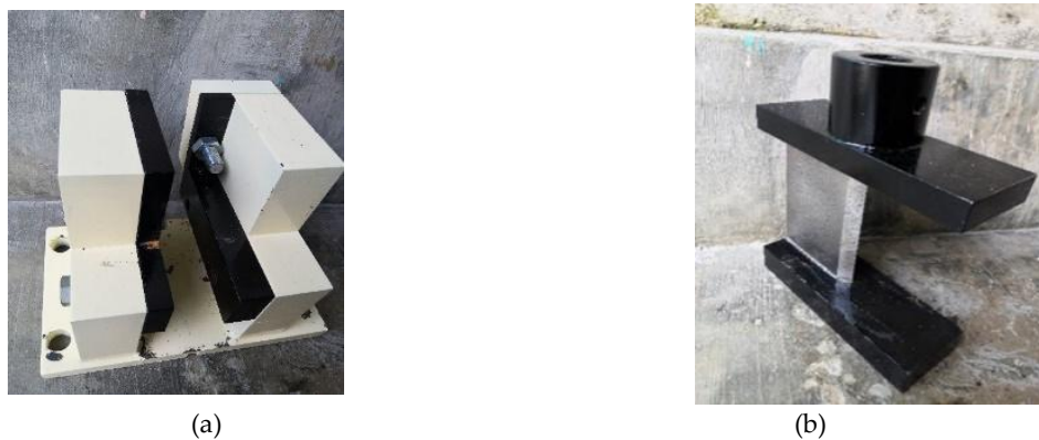
Figure 1. The results of the modifications are as follows: (a) Holder Modification and (b) Pendulum Manufacturing Outcome.
