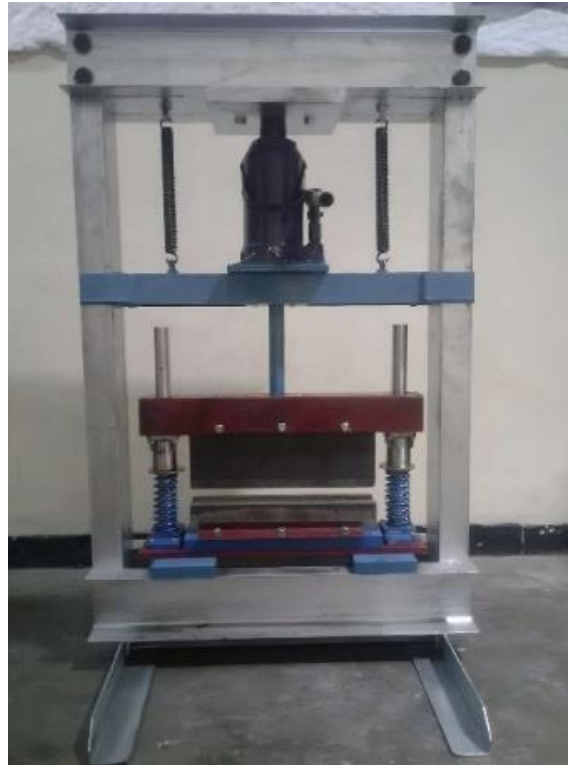
Figure 1. Development of a Portable Bending Device with a Hydraulic Jack System[6].
