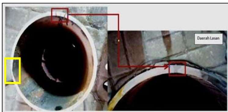
Figure 4. The HAZ Area Did Not Experience Failure/Thinning
