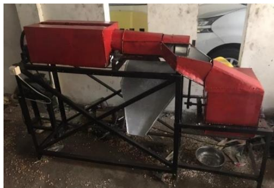
Figure 2. Husker, sheller, and corn cob crusher machine design
