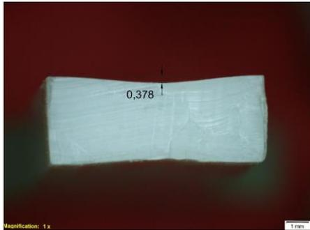
**Gambar 2.** Foto Optik Makro HDPE Daur Ulang Minimum *Sink Marks* percobaan 25
