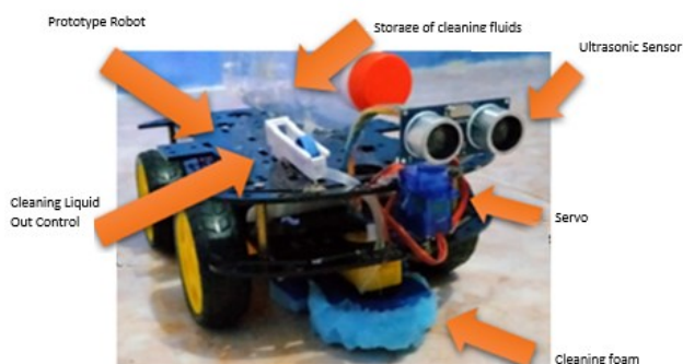
Fig. 6. Automatic Floor Cleaning Robot Prototype detects distance
