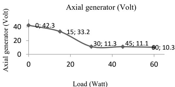
Fig. 10. Axial generator load voltage graph.
