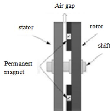
Fig. 4. Axial air gap generator
