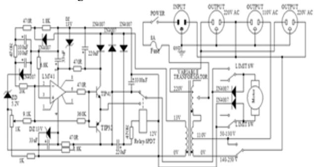
Fig. 8. Automatic Voltage Regulator (AVR) Circuit Scheme.
