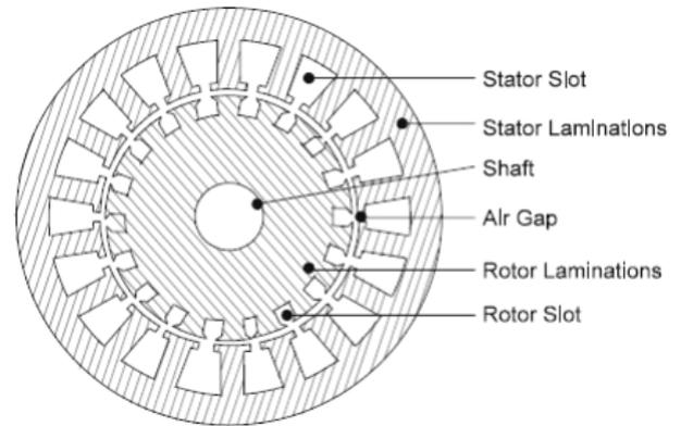
Fig. 3. Stator design
