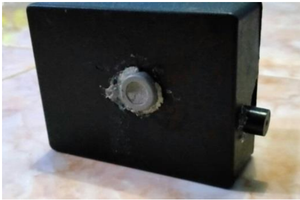
Fig.2. Implementation of LPG Gas Leak Detector System Testing
