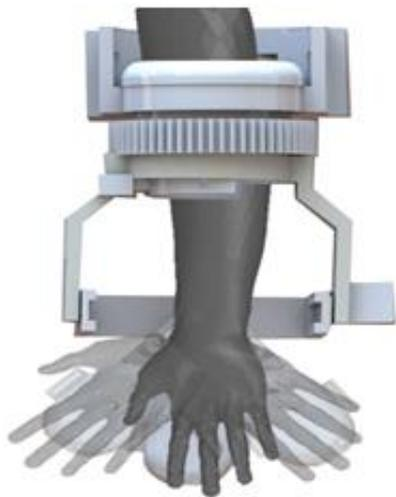
Fig. 12. Adduction and Abduction Movement of the Exoskeleton.
