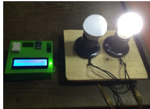
Fig. 10. Testing the SSR circuit on SSR2 in HIGH. Conditions
