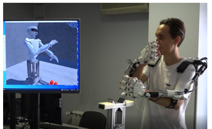
Fig. 11. Manipulator self-collision blocking on the robot SAR-401 simulator
