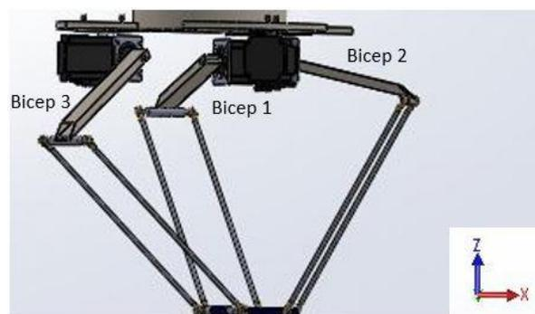
Fig. 8. Labelled bicep of a delta robot arm.
