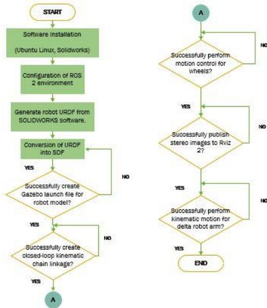
Fig. 1. The flow chart of the simulation development
