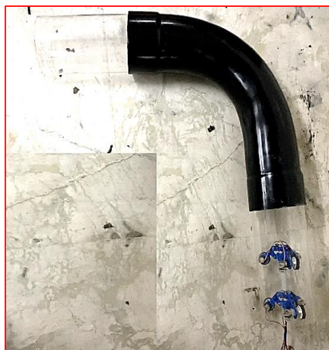
Fig. 28. Robot moving through the experimental setup
