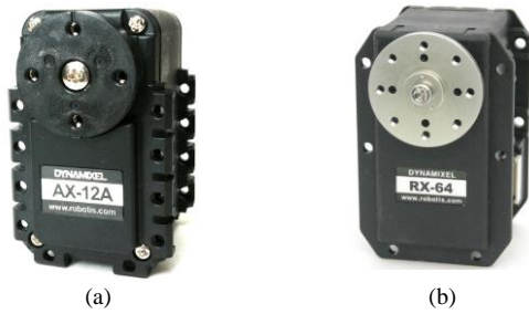
Fig. 5. Servomotors used (a) dynamixel AX 12 A (b) dynamixel RX-64
