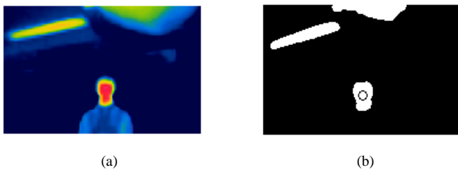
Fig. 9. Face recognition by the roundness (a) Thermal camera detection of a face (b) detected face using circularity
