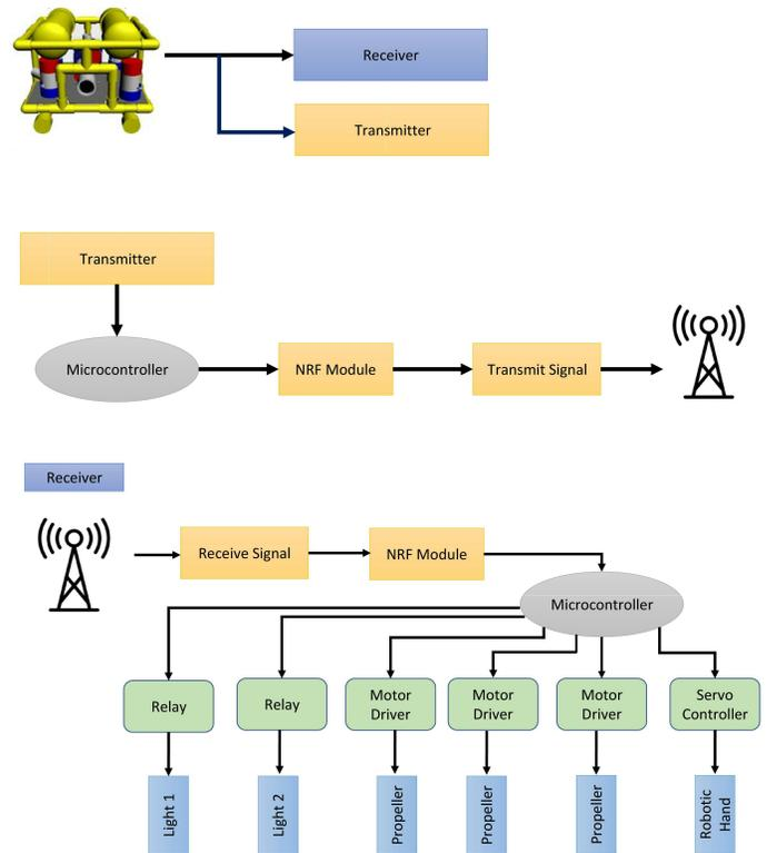
Fig. 1. Block diagram of the proposed underwater drone.
