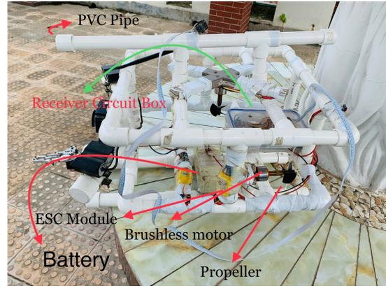
Fig. 7. Side view of the implemented underwater device.
