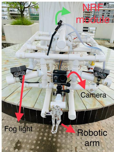
Fig. 6. Front view of the proposed underwater drone.
