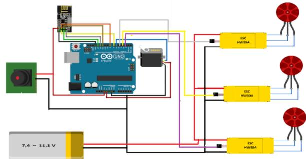
Fig. 11. Circuit diagram of the receiver circuit.
