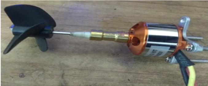
Fig. 9. Brushless motor with the propeller.
