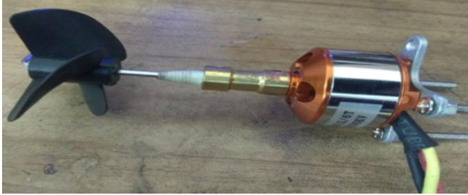
Fig. 9. Brushless motor with the propeller.
