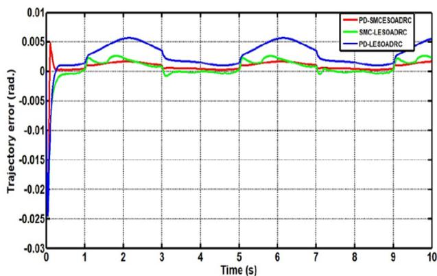
Fig. 6. Comparison of trajectory error results of the three controllers based ADRC without disturbance
