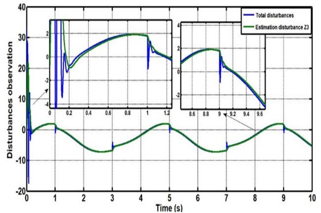
Fig. 8. Shows total disturbance (internal dynamic effects) and its estimation
