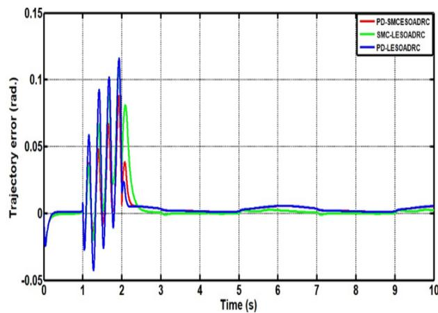
Fig. 10. comparison of trajectory error results of the three controllers based on ADRC with noise disturbance
