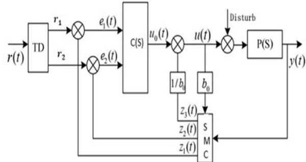
Fig. 3. Show ADRC-based SMC structure
