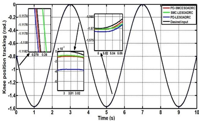
Fig. 5. Simulation results of the three controllers based ADRC without disturbance
