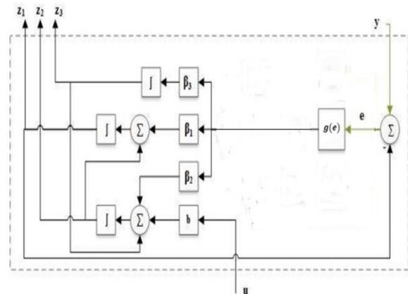
Fig. 4. Show the details of the SMCESO structure
