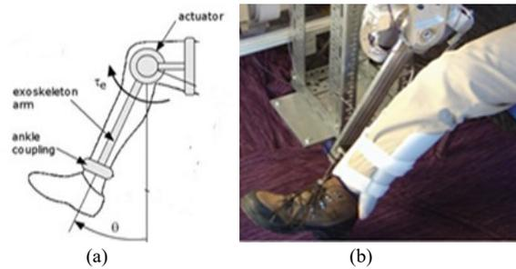
Fig. 1. 1-DOF exoskeleton coupled to a subject's leg, (a) schematic diagram, (b) Practical diagram
