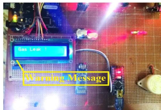
Fig. 10. Appeared message in case of gas leak
