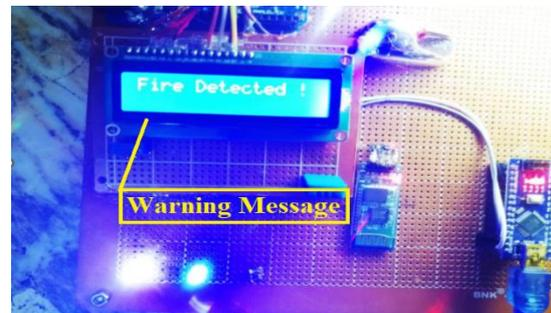
Fig. 9. Appeared message in case of fire detection
