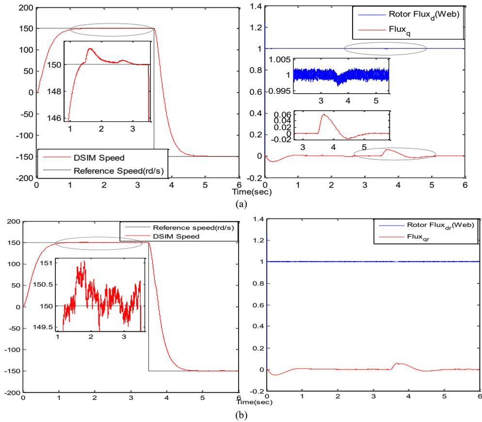
Fig. 4. Parameter variation of +50%Rr; for nominal speed test. (a) proposed state observer. (b) SM-MRAS estimator [32].
