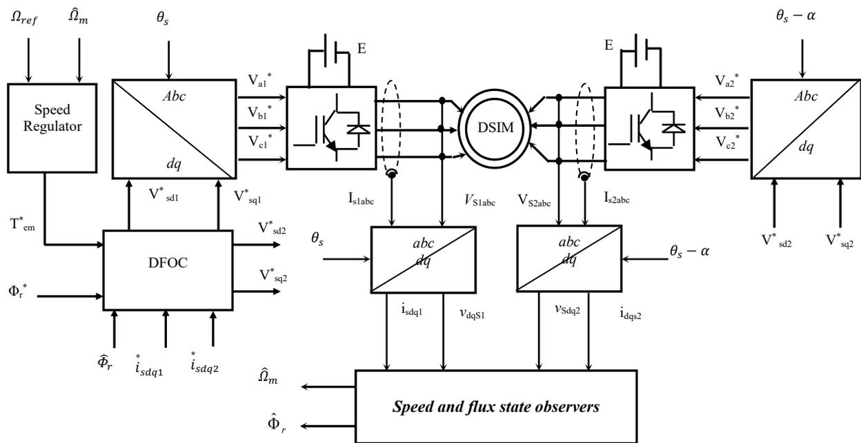
Fig. 1. Sensorless vector control scheme of DSIM
