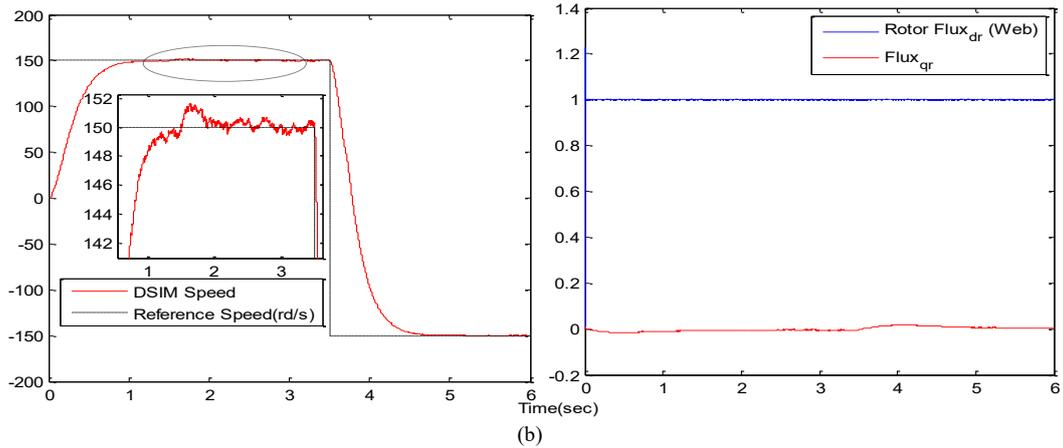
Fig. 8. Parameter variation of -50% Lm; for nominal speed test (a) proposed state observer (b) SM-MRAS estimator [32].
