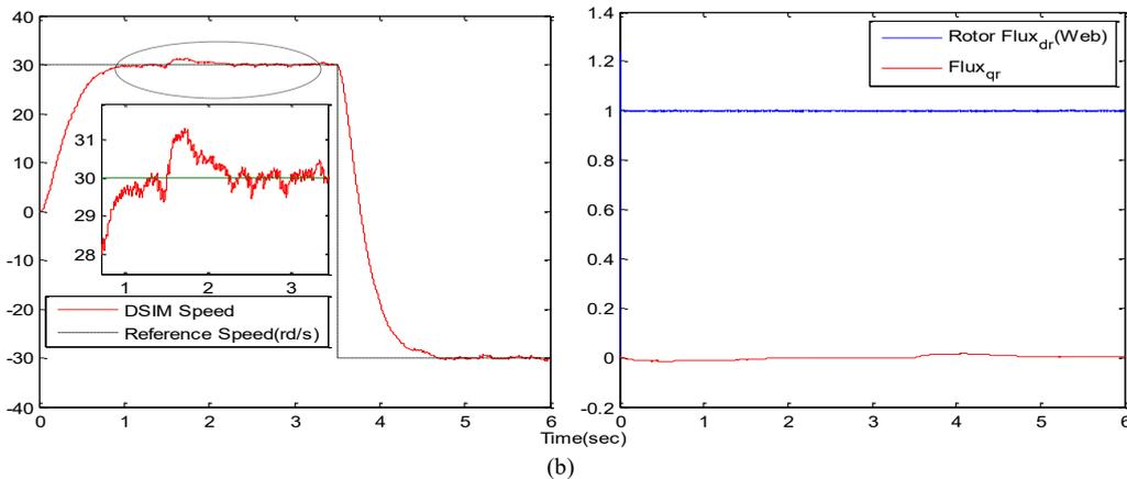
Fig. 9. Parameter variation of -50% Lm; for a low-speed test (a) proposed state observer (b) SM-MRAS estimator [32].
