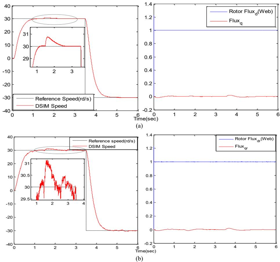
Fig. 5. Parameter variation of +50%Rr; for a low-speed test (a) proposed state observer (b) SM-MRAS estimator [32].
