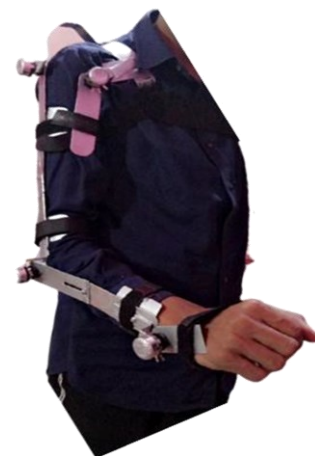
Fig. 2. Arm wearable device (Master). The research team member has worn the device.
