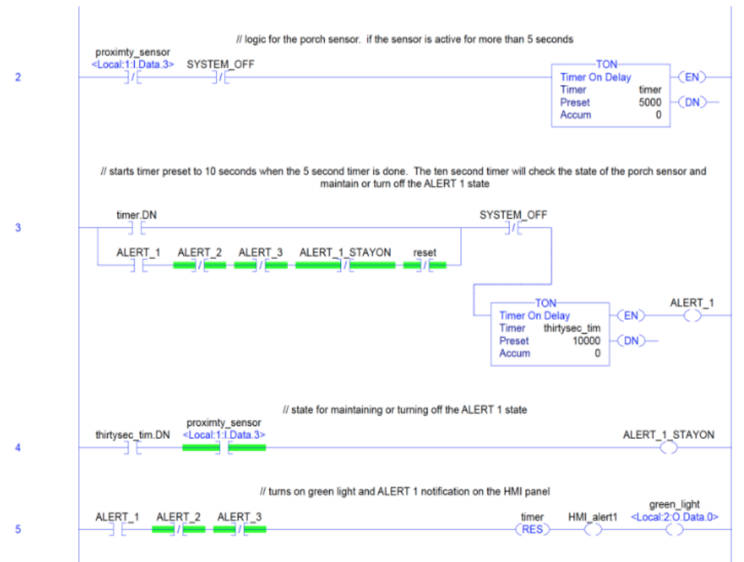
Fig. 6. The second part of ladder logic program for the PLC and field device interface for the controller of the home security system.
