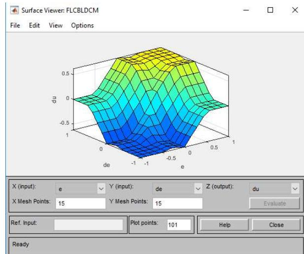
Fig. 11. The FLC-Surface viewer of input (e, de) & output (du)
