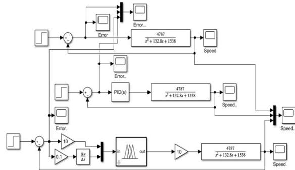
Fig. 4. Model of BLPMDC motor without a controller, with PID controller, and with FLC
