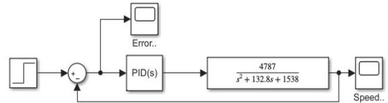
Fig. 2. Model of BLPMDC motor with PID controller
