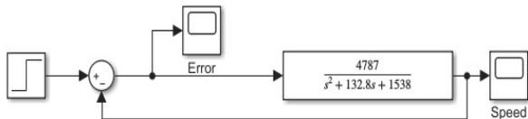
Fig. 1. Model of BLPMDC motor without controller
