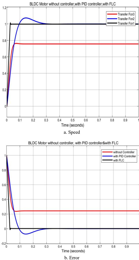
Fig. 15. Simulation response of the motor without the controller, with PID controller, and with FLC
