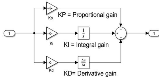
Fig. 5. PID controller
