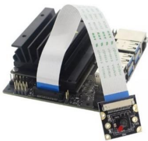
Fig. 8. Jetson nano with 8MP Sony IMX219 77-degree CSI camera
