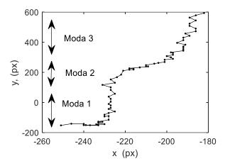
Fig. 6. The movement trajectory of the cube center and three different modes in the image plane coordinates
