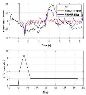
Fig. 8. Dependencies the one-step prediction estimation errors for the model state and the horizon sizes on time
