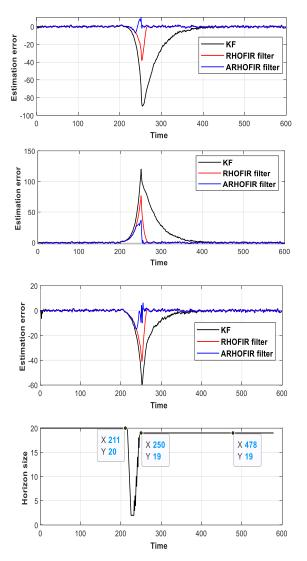
Fig. 3. Dependensies estimation errors for the model state and the horizon sizes on time
