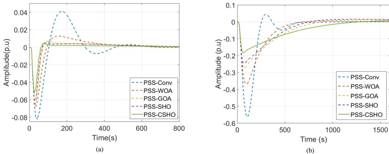
Fig. 5. Transient Response of Case Study 2 (a) Speed Response (b) Rotor Angle Response
