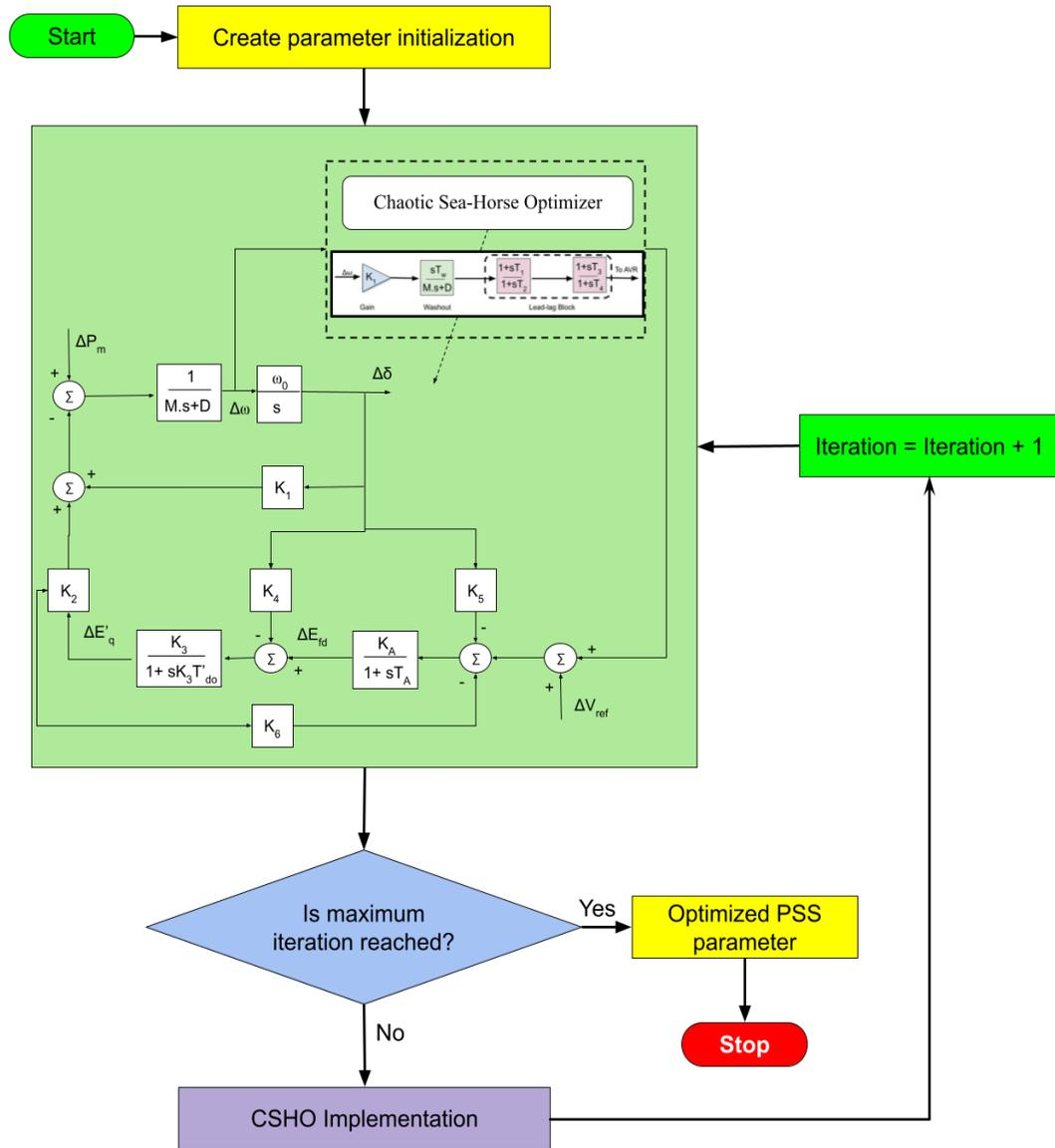
Fig. 2. Block diagram of the proposed CSHO algorithm implementation on PSS Lead-Lag.
