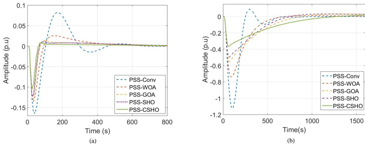
Fig. 4. Transient Response of Case Study 1 (a) Speed Response (b) Rotor Angle Response
