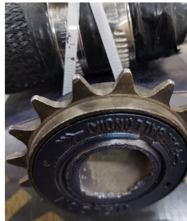
Fig. 8. The freewheel to obtain unidirectional moving
