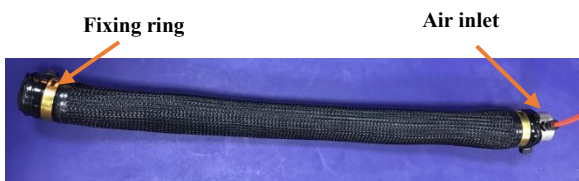
Fig. 4. The constructed pneumatic artificial muscle
