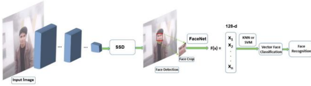
Fig. 14. FaceNet model based on MobileNetV2 backbone and SSD subsection
