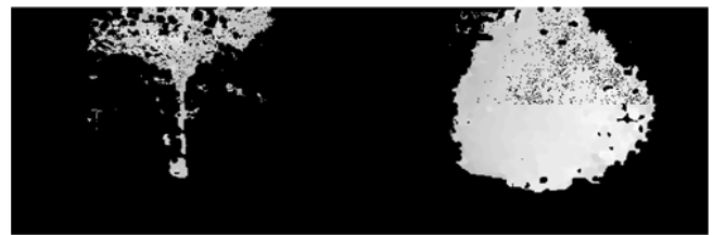
Fig. 21. Obstacle disparities extracted from the u disparity image
