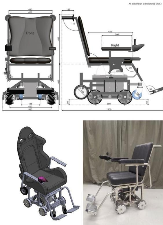
Fig. 7. The electric wheelchair with mecanum wheel.
