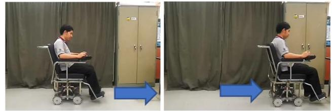
Fig. 23. Forward testing of the electric wheelchair.
