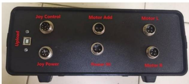
Fig. 2. Controller box of the electric wheelchair
