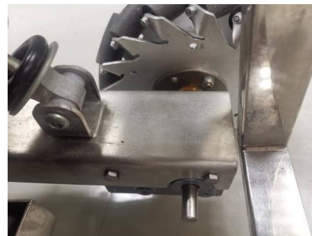
Fig. 10. Assembling the motor part of the electric wheelchair.
