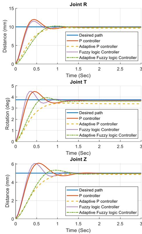
Fig. 20. Results of the step input value system simulation in Test 1.
