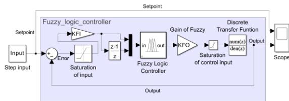
Fig. 17. The program in Simulink that uses fuzzy logic control to control the system.
