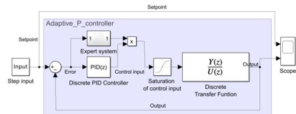
Fig. 7. The Simulink diagram of the Adaptive P Controller is shown in the form of a block diagram.
