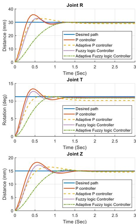
Fig. 21. Results of the step input value system simulation in Test 2.
