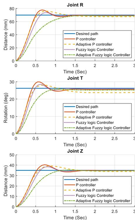
Fig. 23. Results of the step input value system simulation in Test 4.
