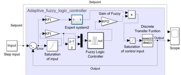
Fig. 19. The program in Simulink that uses adaptive fuzzy logic control to control the system.
