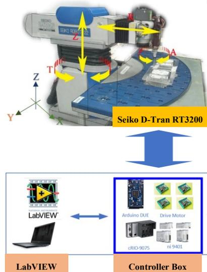
Fig. 3. Seiko D-Tran RT3200 and device for controller.
