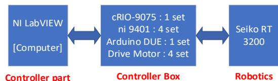
Fig. 4. Block diagram of the overall system.
