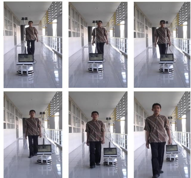
Fig. 33. The robot process avoids obstacles when the object is straight in front of the robot
