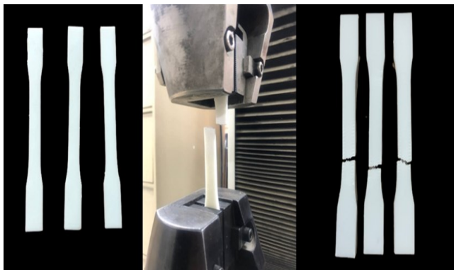
Fig. 11. Tensile Test Specimens before and after a fracture
