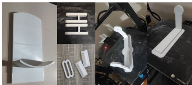
Fig. 5. Printed parts of the exoskeleton
